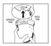
c. Line up the green and red tabs with the green and red labels. Push in on the tabs. Insert the side with the green tab, then the side with red tab. Continue pushing on the ends of the tabs until both sides click into place.
